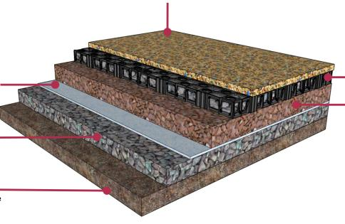
**SureCell** (Installed by SureSet or others) 52mm depth fully connected cellular reinforcement structure infilled with well compacted 4/10mm graded crushed aggregate to BS EN12620
